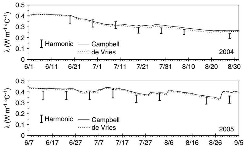
Figure 7. Thermal conductivity estimated by applying the harmonic method for 10-day periods, assuming  $\Delta z = 4.75\text{--}5.25$  cm. Continuous lines indicate daily values of thermal conductivity estimated by the equations of Campbell *et al.* (1994) and de Vries (1963)
