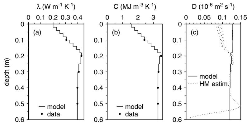
Figure 5. Profiles of (a) thermal conductivity, (b) volumetric heat capacity, and (c) thermal diffusivity. Solid circles in (a) and (b) indicate estimated values based on the average soil temperature and moisture content data in June 2005. Solid lines indicate the values used in numerical simulation. Dashed line in (c) indicates the diffusivity values calculated from simulated amplitude of fluctuation using the harmonic analysis (HM)
