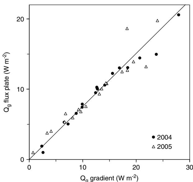
Figure 8. Comparison of 5-day average ground heat flux ( $Q_g$ ) measured with the heat flux plate and estimated by the gradient method
