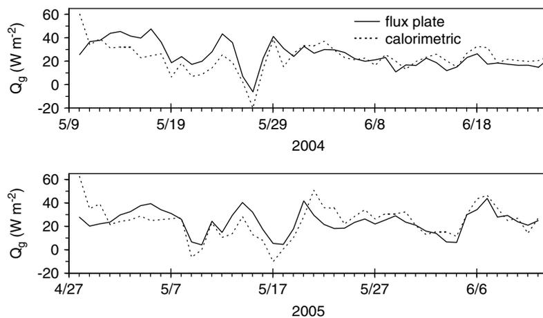
Figure 9. Comparison of the ground heat flux ( $Q_g$ ) measured by the flux plate and the calorimetric method
