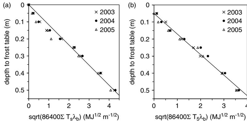
Figure 11. Relation between the frost table depth and the cumulative product of bulk thermal conductivity ( $\lambda_b$ ) and; (a) surface temperature ( $T_s$ ), (b) soil temperature at 0.05 m ( $T_5$ ). Solid lines show Equations (4) and (16) with the least-squares fit values of  $\alpha$
