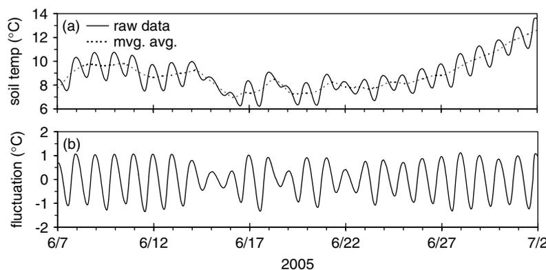
Figure 6. (a) Raw soil temperature data and 24-h moving average at 0.2 m depth in June 2005. (b) De-trended data given by the difference between the raw data and the moving average
