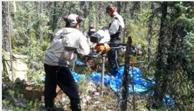
Installing deep temperature sensors in the forested area which exists only above permafrost areas, which have been retreating in some spots at a metre per year. © Courtesy W Quinton
