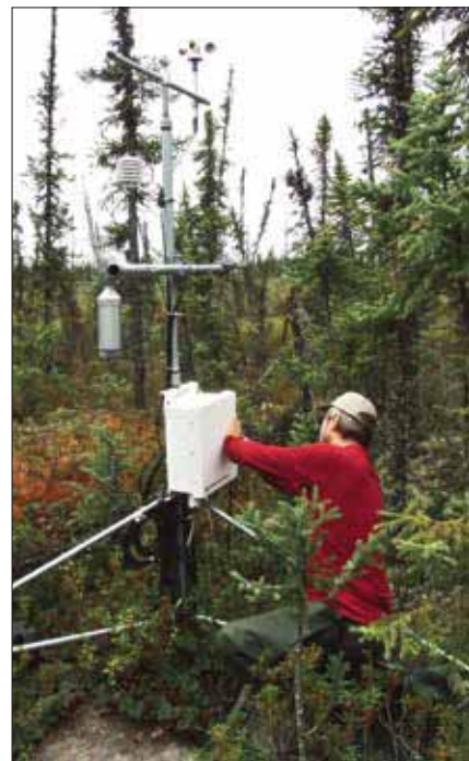
Bill Quinton, who founded the Scotty Creek research site, changes a storage module in a data logger that records information from instruments measuring snow depth, wind speed, and short- and long-wave radiation.
